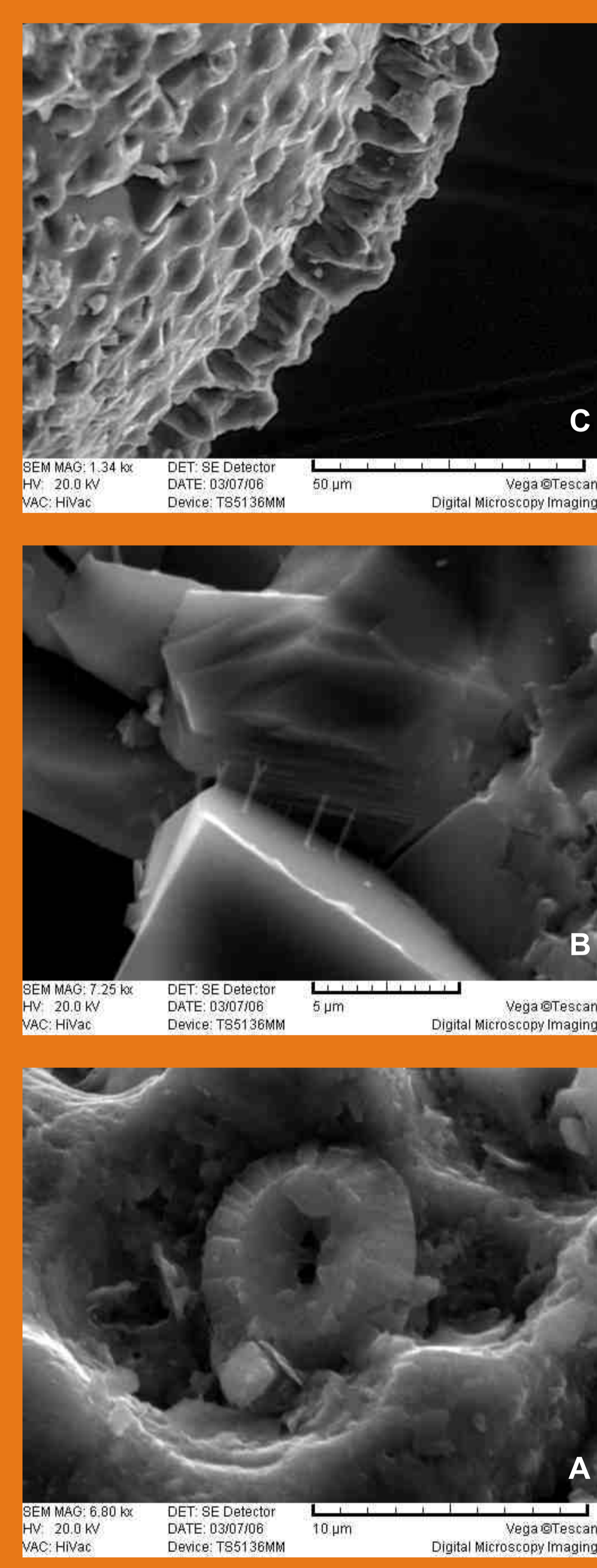
Fig. 3. Diagenetic mineralization processes were investigated by a Tescan TS 5136 SEM microscope equipped with an Oxford energy dispersive spectrometer in a Electron microscope laboratory, Faculty of Science, Department of Geology, Zagreb.
