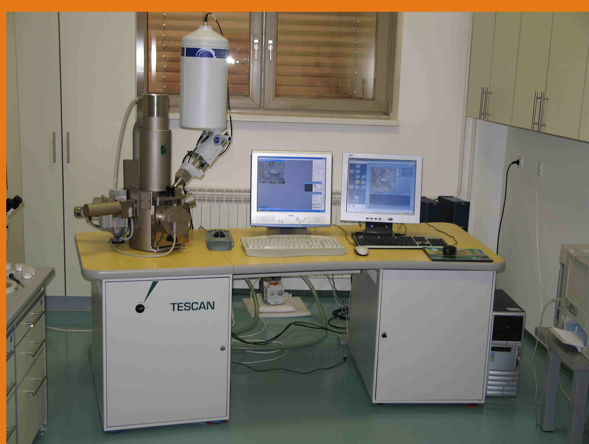
Fig. 3. Diagenetic mineralization processes were investigated by a Tescan TS 5136 SEM microscope equipped with an Oxford energy dispersive spectrometer in a Electron microscope laboratory, Faculty of Science, Department of Geology, Zagreb.
