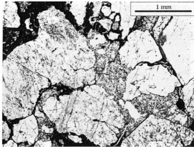
Fig 6 Stop 2. Permian sandstone from Opaljenac quarry with barite-pyrite mineralization in the intergranular pores.
